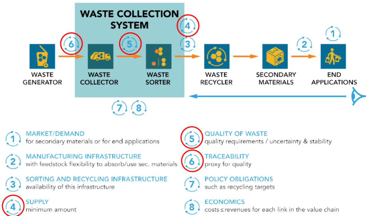
Figure 12: main requirements for the waste recycling value chain to enable the production of more value through the generation of secondary raw materials. The main requirements for waste collection systems are highlighted in red (Source: COLLECTORS, D2.2)
