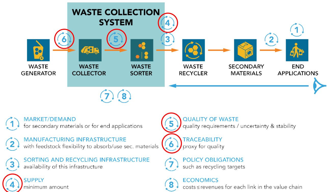
Figure 9: Boundary conditions for recycling related to the waste collection system, indicated in red
